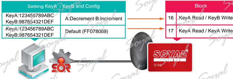
Setting KeyA / KeyB and Config in MIFAREKEY software and write to SIM card block 16 and block 17
