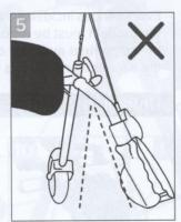
The position of the locking lever itself can be adjusted by simultaneously pulling and rotating it. To change the height setting of the push handles, rotate the locking lever counterclockwise in order to release the fixation. Then lock the handle at the desired height, as described above.
