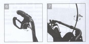
If braking is poor or too hard, the brake can be adjusted either at the brake housing above (**pic. 6**) or using the adjusting screw on the Bowden cable below (**pic. 7**) to achieve the desired braking effect. The brake is correctly adjusted when the brake lever as well as the brake wires are free of play and the wheels can be rotated without grinding noises when the brake is released.
