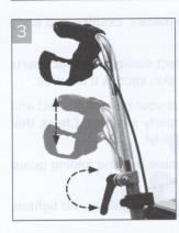
Insert push handles at least to the "**MAX**" mark in the frame tube (**pic. 3**). Secure them at the desired height by turning the locking lever clockwise. Adjust both handles to the same height.
