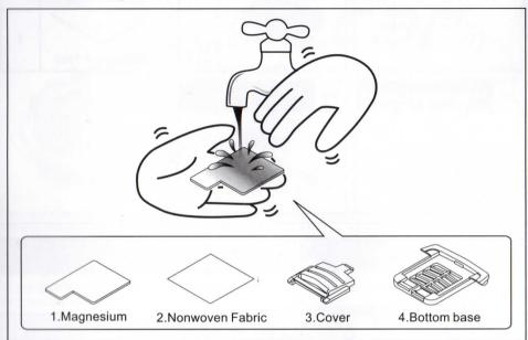
When car is getting slow or stop, suck salt water and add few drops into the position as shown on the left, don't drop into the polarity of connectors to avoid oxidization.
