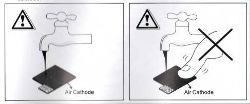
• Flush below parts and hand rub the surface, make sure no salt residue. Dry all parts separately. (Important: If salt is residual on the magnesium sheet, it will shorten it's life.)
